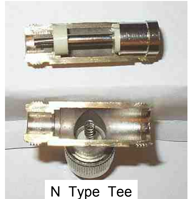
N Type Tee CENTER CONNECTOR USES A SPRING FOR CONTACT !
