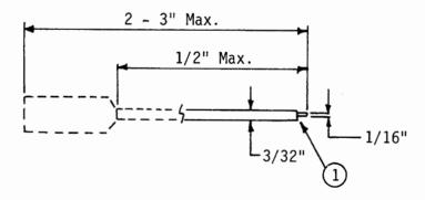
1 Blade must be narrower than 3/32" insulated shank so as not to create metal shavings from blade scraping on inner threaded barrel of capacitor.
