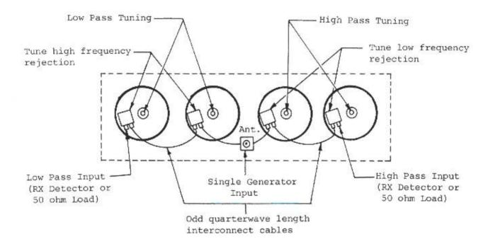
NOTE: Low Pass Input on left of unit is strictly a convenient convention.
