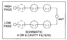
The duplexer is tuned using either test setup as shown in Figures 1 or 2. It is recommended to use a 6-10 dB, 50 OHM pad in the input lines in order to reduce VSWR reflections which may be introduced in the test equipment being used. (refer to CI-1070)
