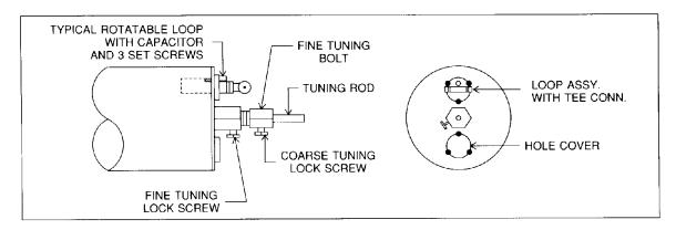
The duplexer is tuned using either test setup as shown in Figures 1 or 2. It is recommended to use a 6-10 dB, 50 OHM pad in the input lines in order to reduce VSWR reflections which may be introduced in the test equipment being use. (refer to CI-1070)
